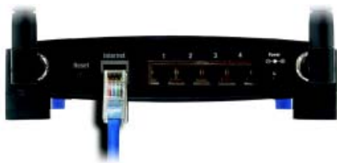
Figure 4-5: Connecting Another Router
