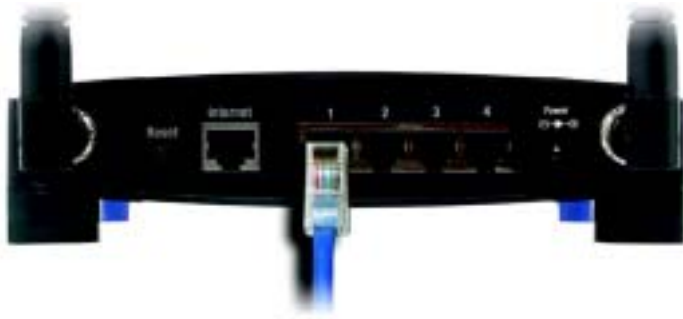
Figure 4-6: Connecting Your Network Devices
