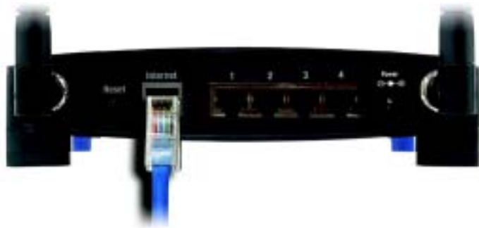
Figure 4-1: Connecting Your Internet Connection
