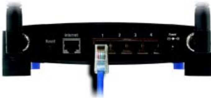
Figure 4-2: Connecting Your Network Devices
