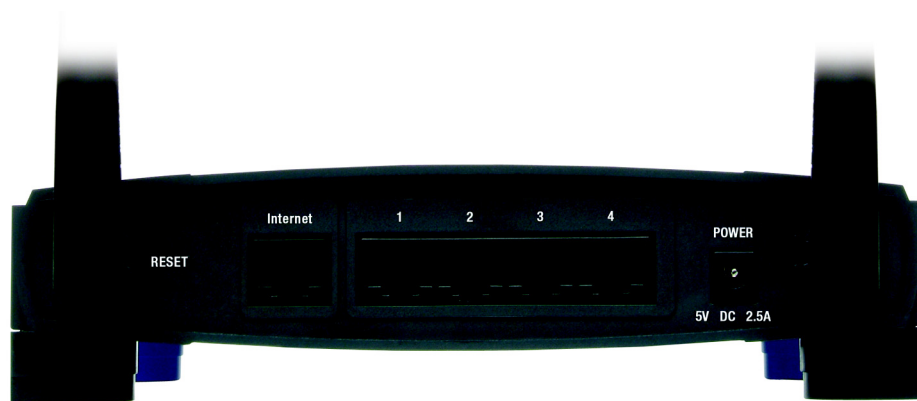
Figure 3-1: The Router's Back Panel
