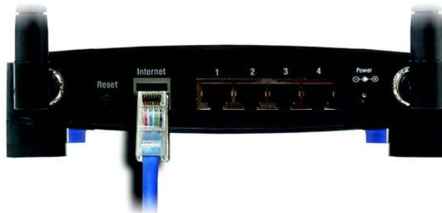
Figure 4-1: Connecting Your Internet Connection
