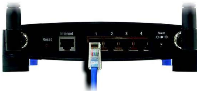
Figure 4-2: Connecting Your Network Devices
