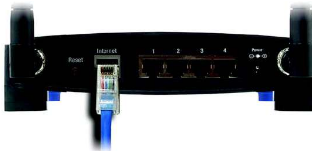
Figure 4-5: Connecting Another Router
