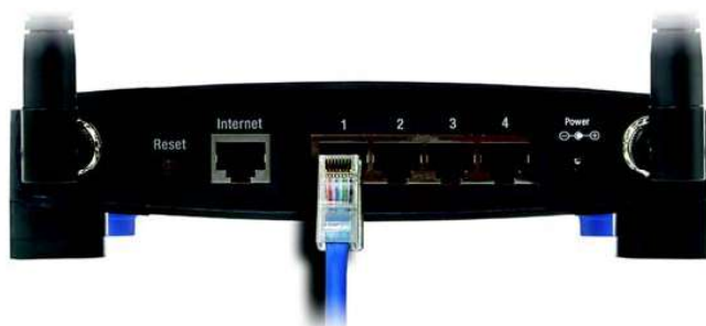
Figure 4-6: Connecting Your Network Devices
