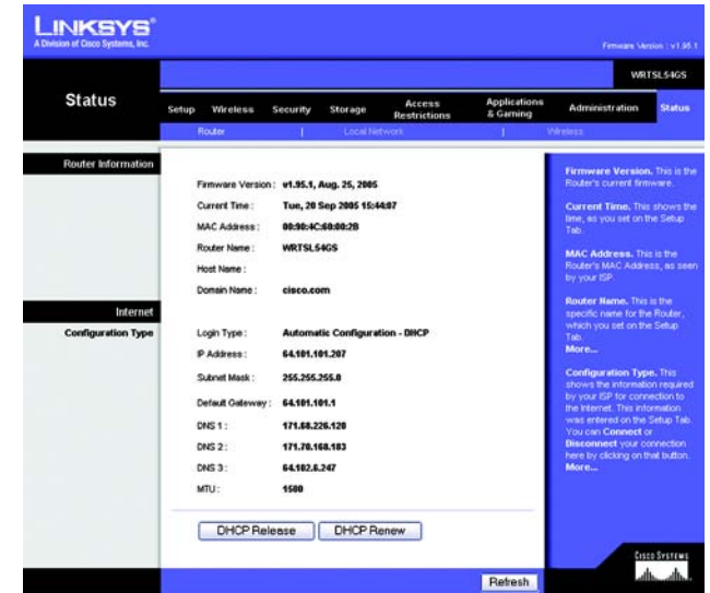
Figure 5-62: Status Tab - Router
