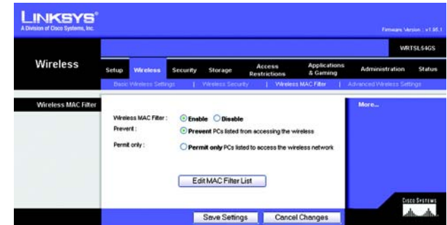
Figure 5-27: Wireless Tab - Wireless MAC Filter
