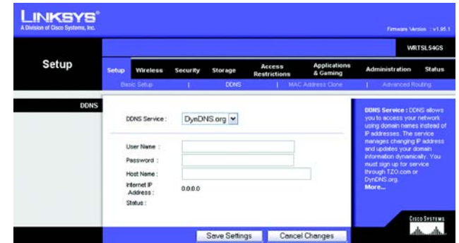
Figure 5-13: Setup Tab - DDNS (DynDNS.org)
