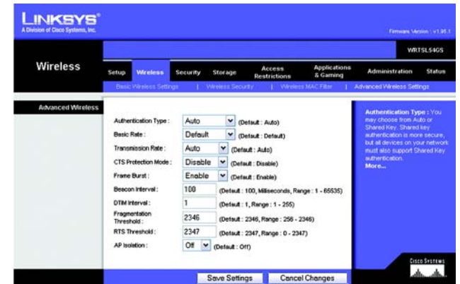
Figure 5-29: Wireless Tab - Advanced Wireless Settings
