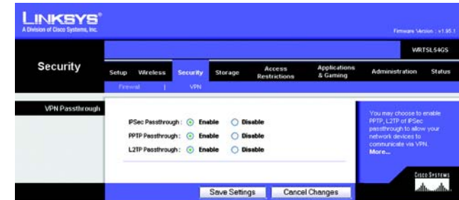
Figure 5-31: Security Tab - VPN Passthrough
