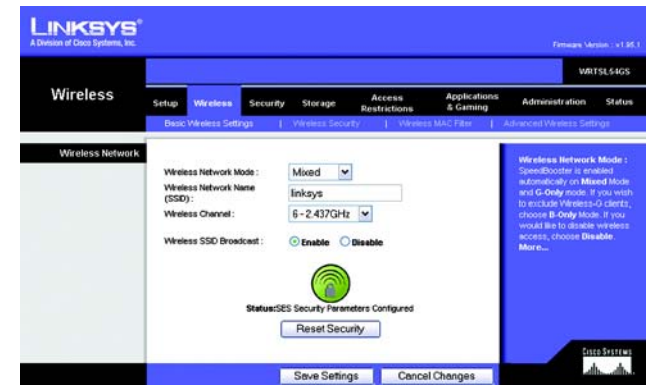
Figure 5-19: Wireless Tab - Basic Wireless Settings
