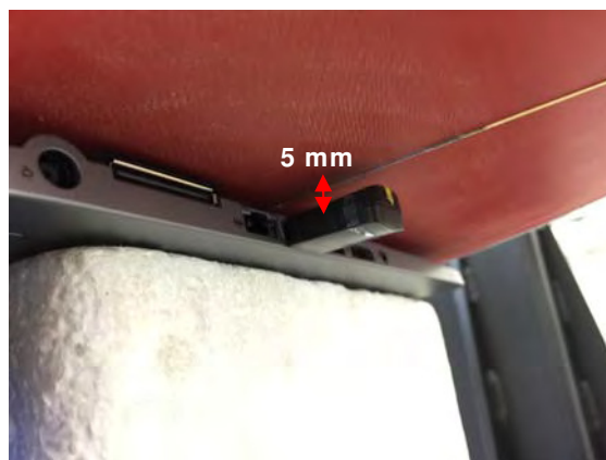
Fig.5 EUT Horizontal-Up to flat phantom
