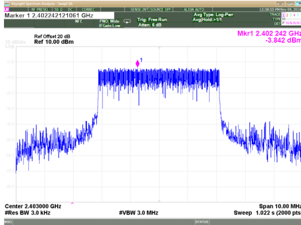
Plot 3.3.4 Maximum Power Spectral Density test results, F_c = 2403\text{MHz} , BW = 4.2\text{ MHz} , Bit Rate = 4 Mbps
