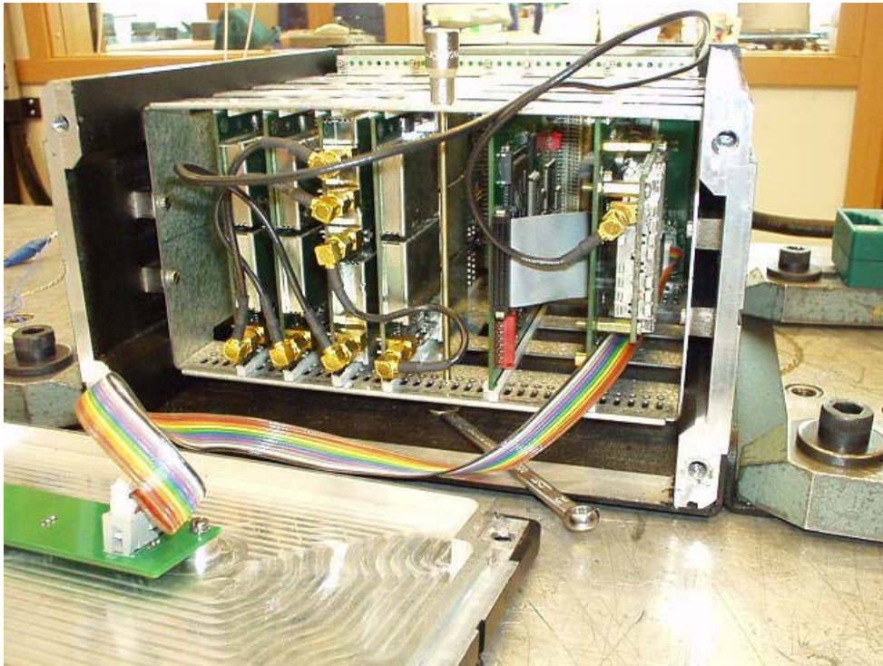
AIS main unit during resonance search test
