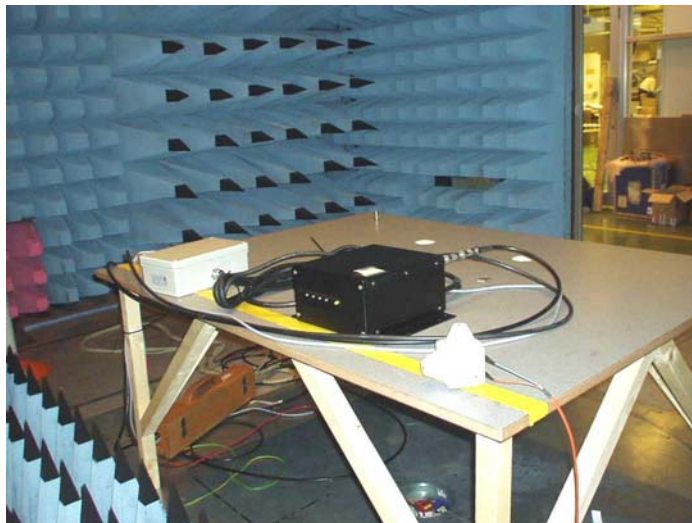
EUT set-up for radiated interference testing
