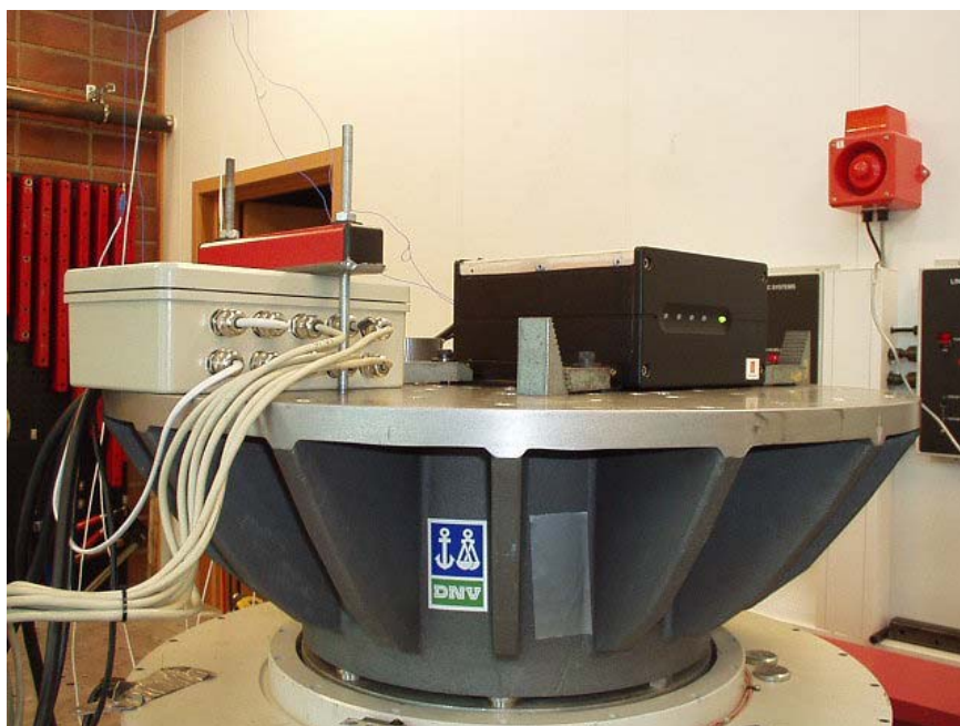
Mounting of EUT items for vibration testing in Z-direction
