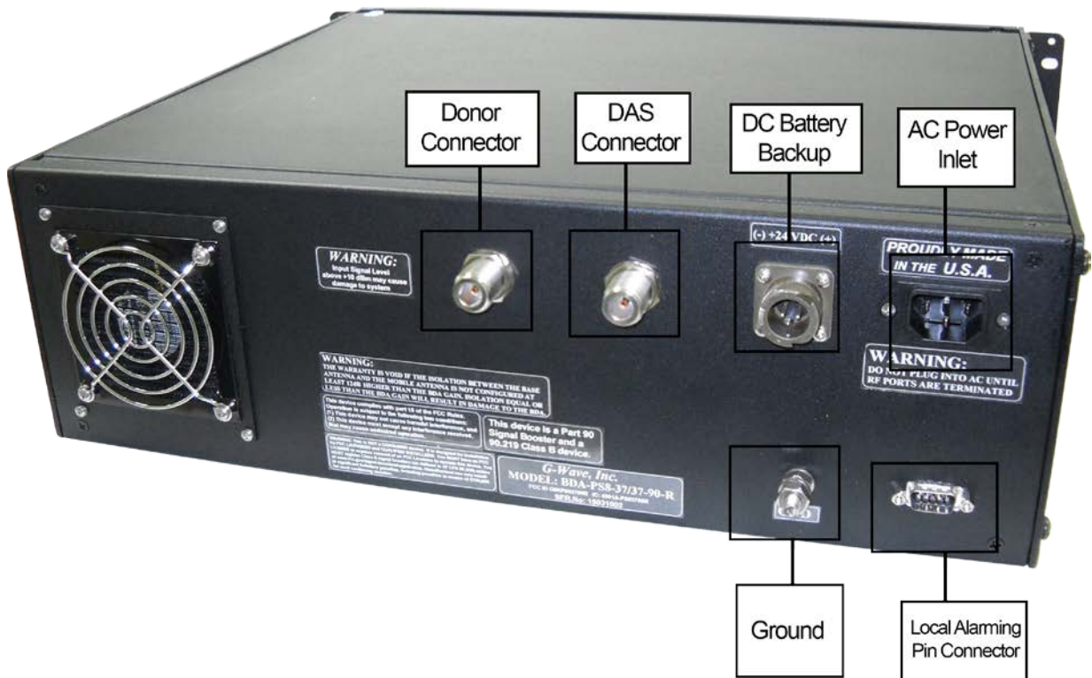
Figure 4: Back Panel Connections
