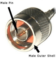
Test for DC short between male pin and outer shell of antenna connectors
