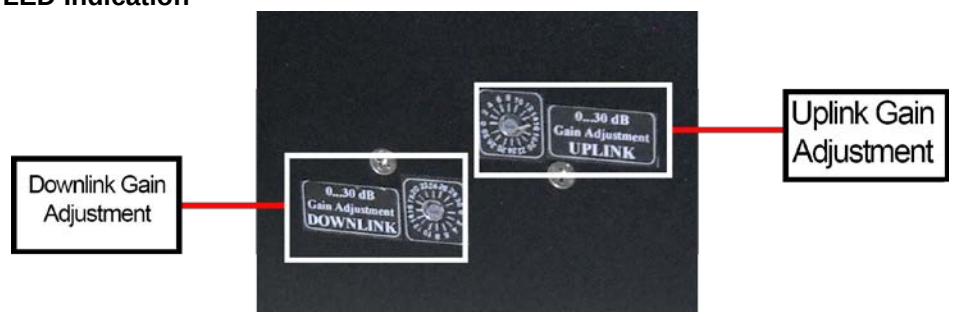
Figure 5b: Front Panel Manual Attenuation In 2 dB steps
