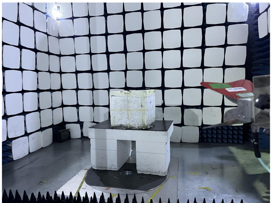
Radiation Emission Test Setup (1GHz to 18GHz)
