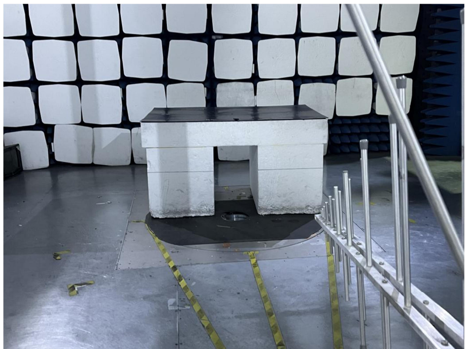
Radiation Emission Test Setup (30MHz to 1GHz)
