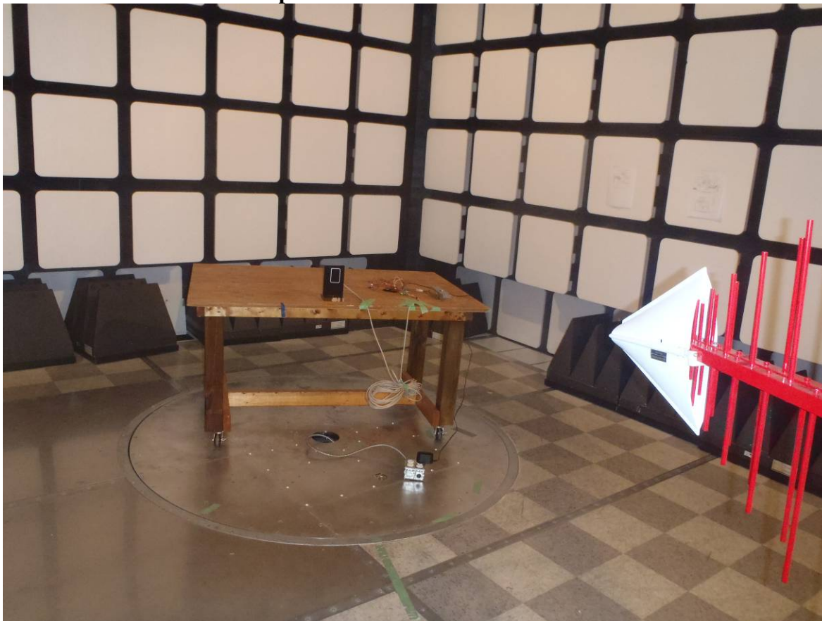
Radiated Emission Test Setup Photo#2:
