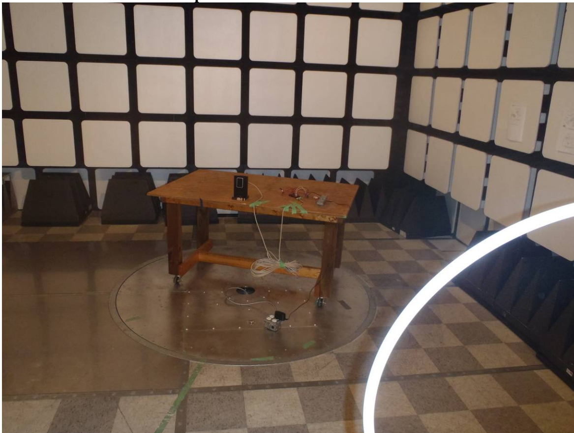
Radiated Emission Test Setup Photo#1:
