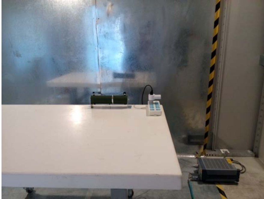
Conducted Emissions - Front View
