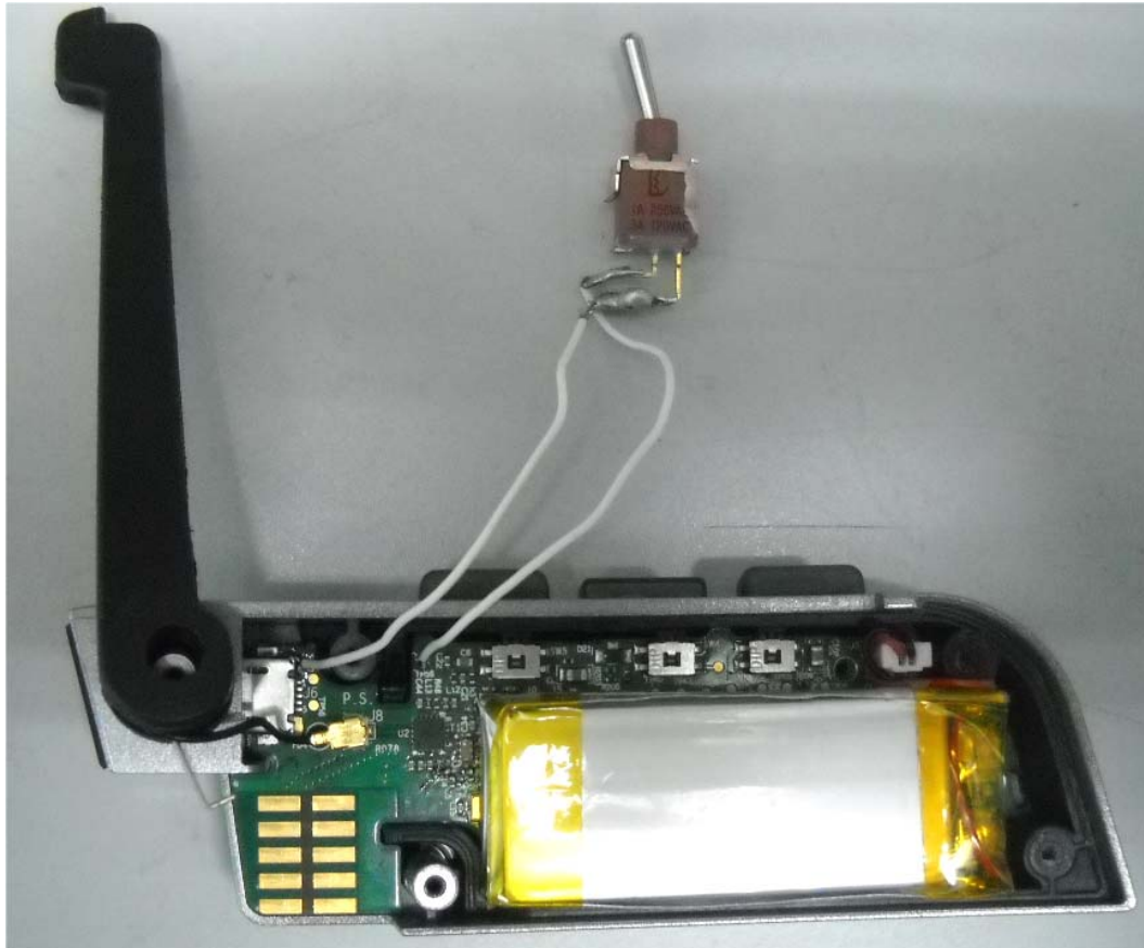
Photograph No.2 Bluetooth headset internal view
