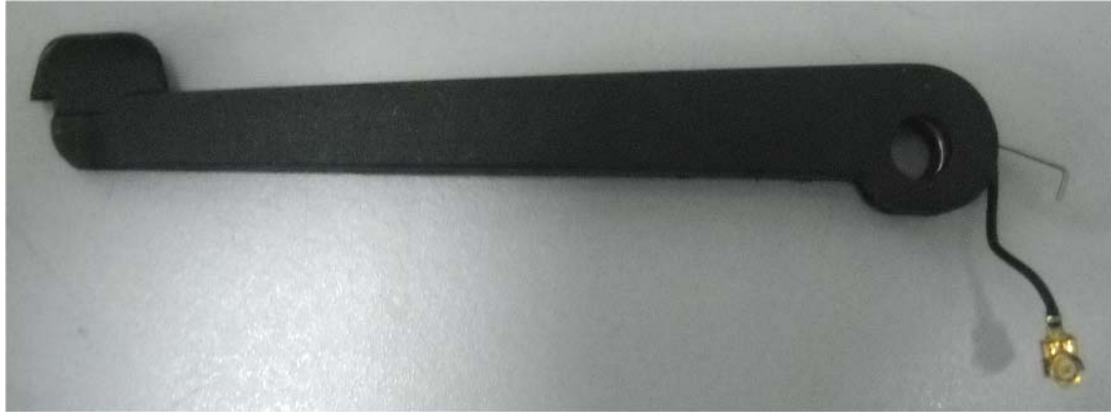
Photograph No.8 Bluetooth headset antenna for operation in 2402-2480 MHz
