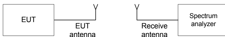
Figure 7.6.1 Band edge emission test setup
