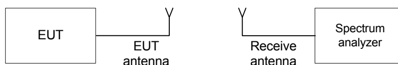
Figure 7.3.1 Hopping frequencies test setup
