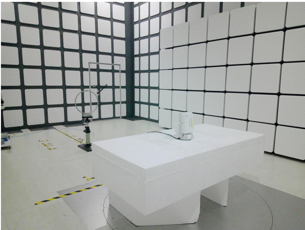
Description: Radiated Emission Test Setup for 9kHz~30MHz_D_ANT
