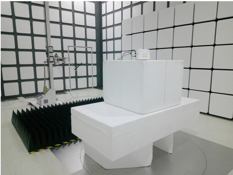
Description: Radiated Emission Test Setup for above 1GHz_ O_ANT
