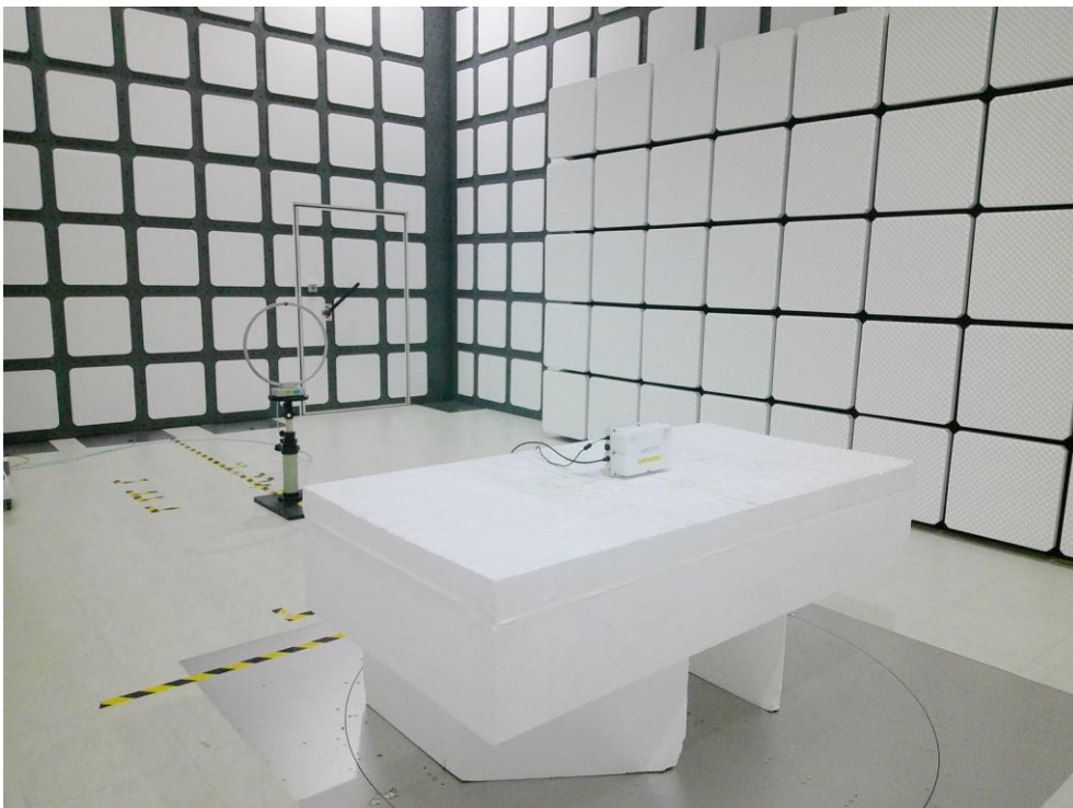
Description: Radiated Emission Test Setup for 9kHz~30MHz_ O_ANT
