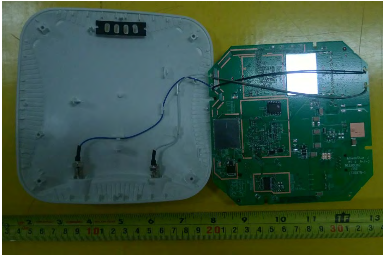
INSIDE OF TOP COVER SHOWING EXTERNAL RF PORTS
