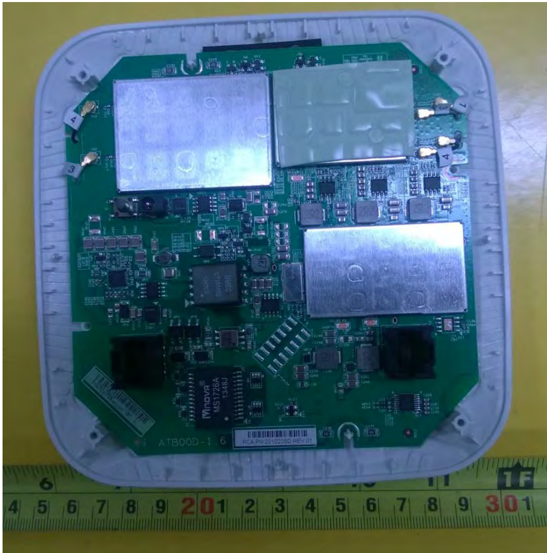
TOP SIDE OF PCB WITH SHIELDS
