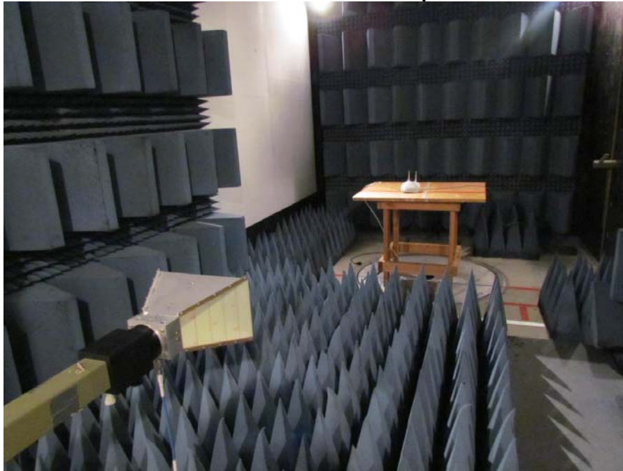
General DFS Test Setup
