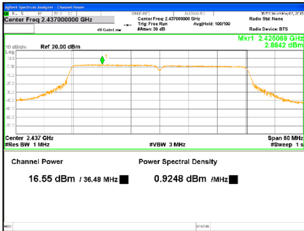
Figure 4: Maximum Transmitted Power, 2437MHz HT40 mode at 13Mbps, Chain 0
