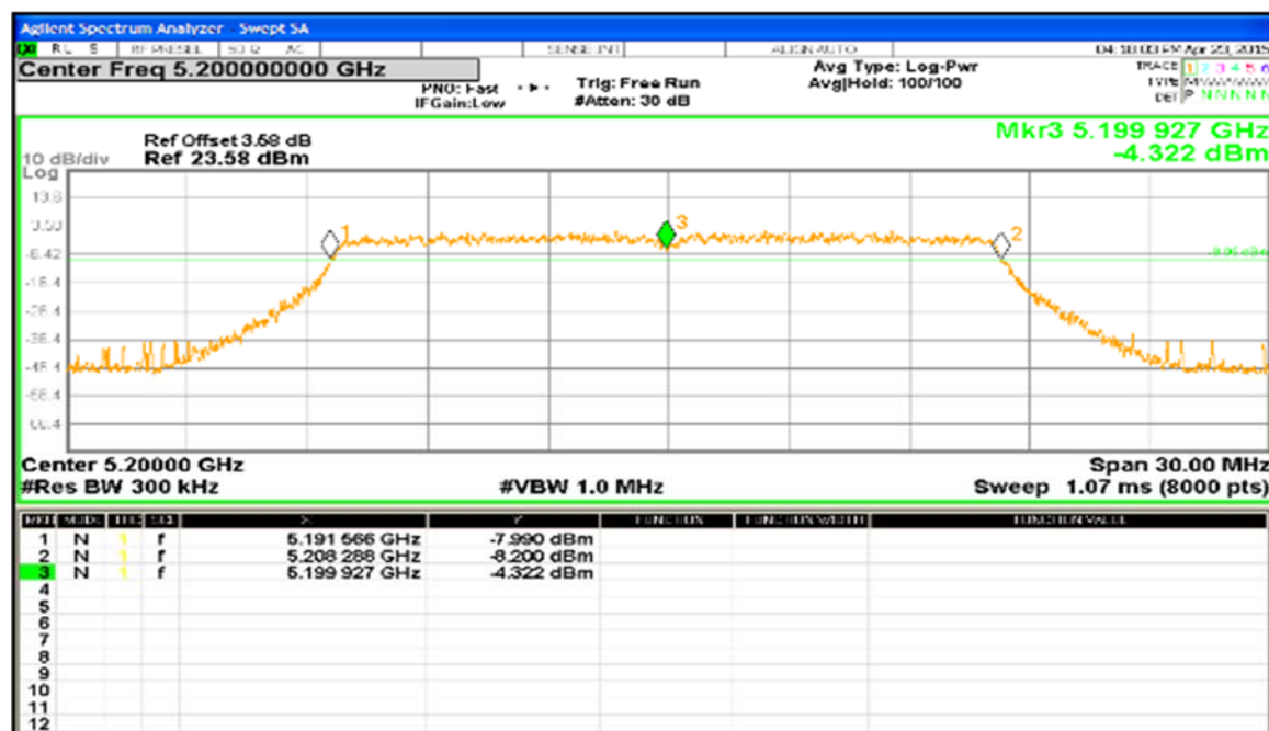
Figure 33: Frequency Stability at 5200MHz 11a mode at 6Mbps
