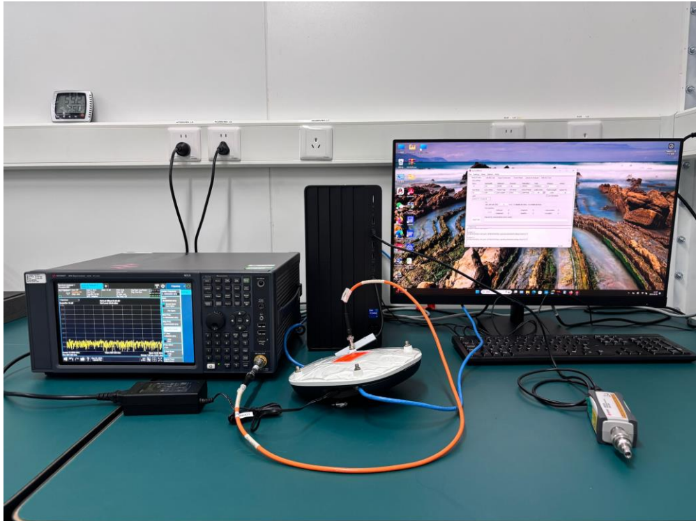
Description: DFS Test Setup for APIN0514
