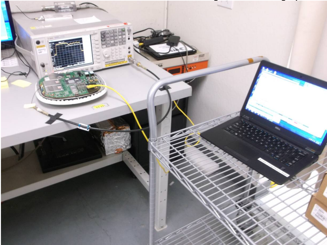
Antenna Conducted Emissions Test Configuration Photographs
