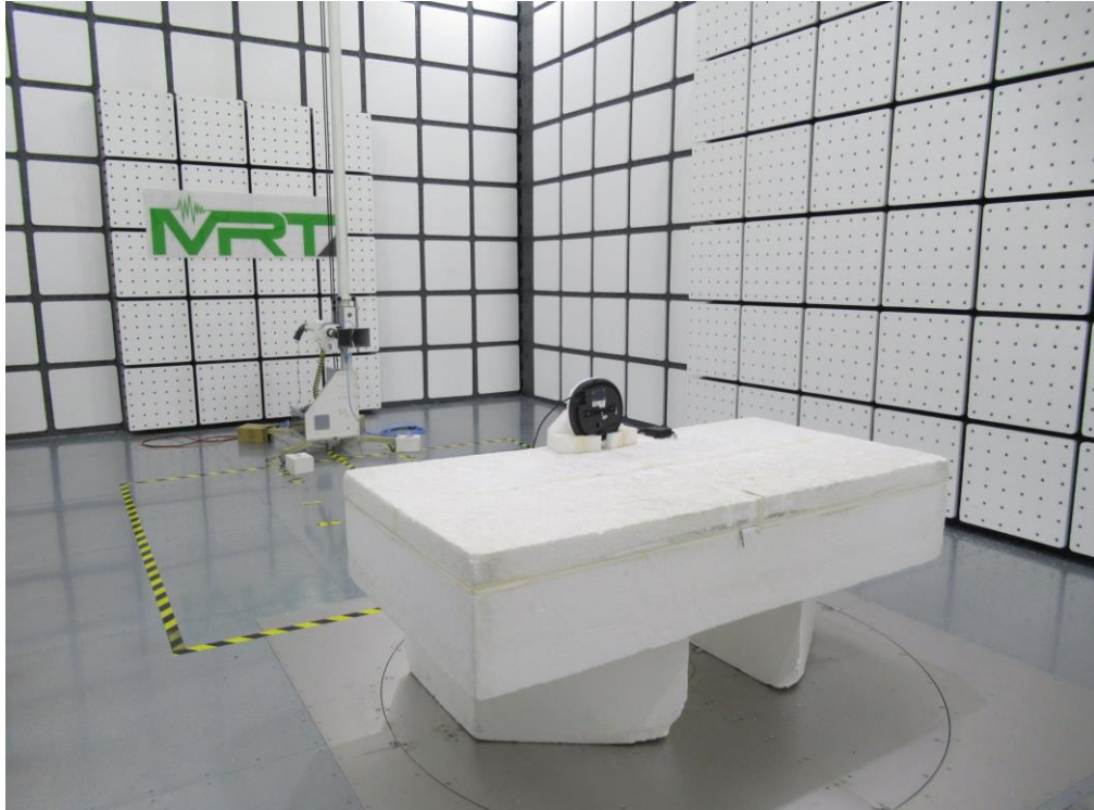
Description: DFS Test Setup _ Radiated
