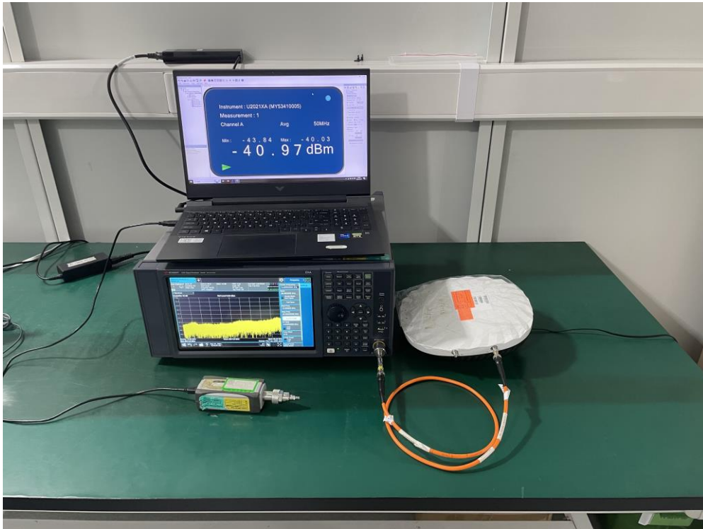
Description: DFS Test Setup
