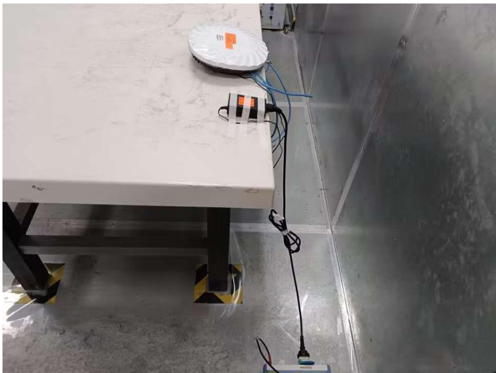
Description: Side View of Conducted Emissions Test Setup for Power Port
