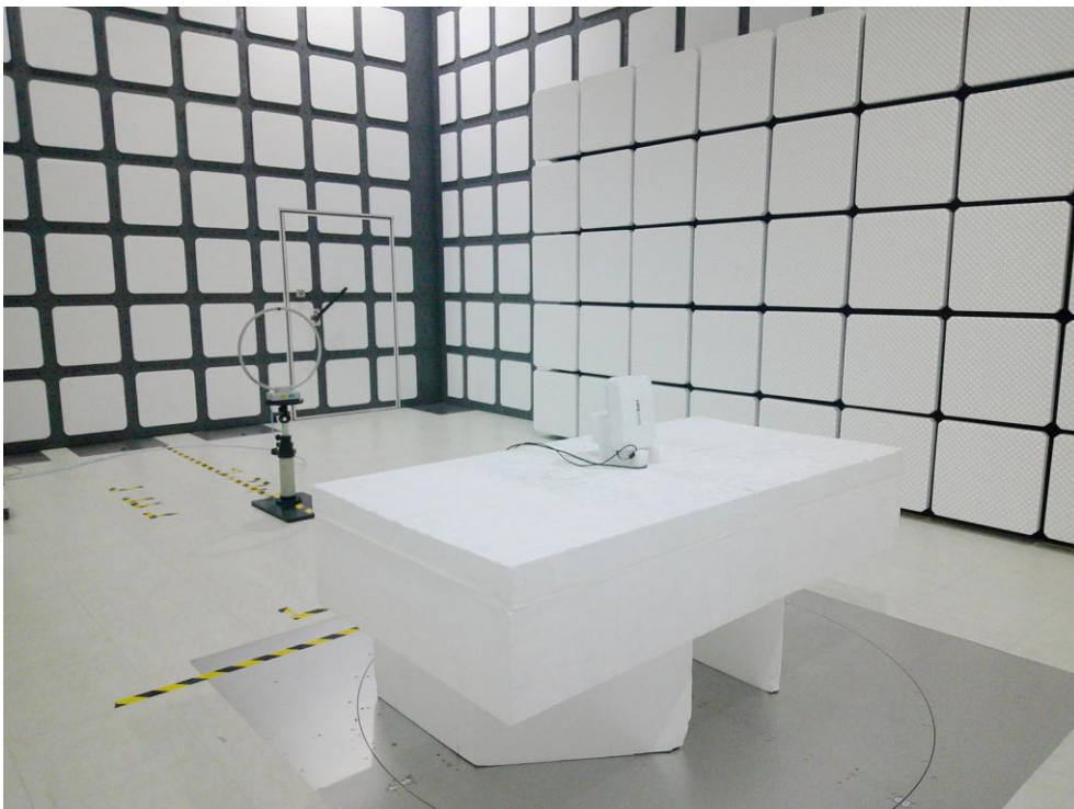
Description: Radiated Emission Test Setup for 9kHz~30MHz_D_ANT
