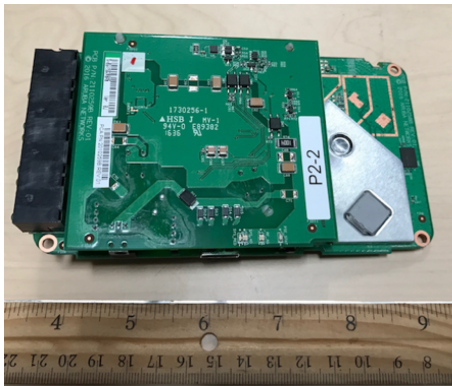
PCB - Antenna Removed
