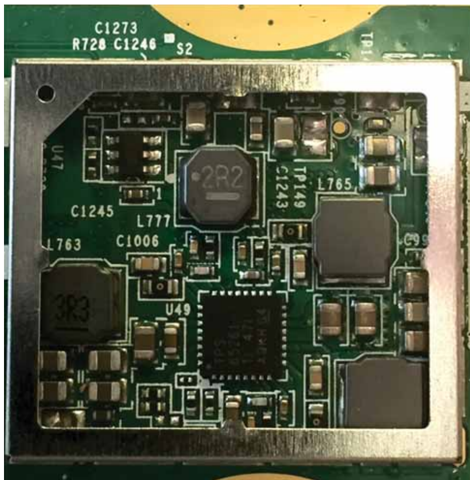
Close-Up of Section Marked 4 – Power
