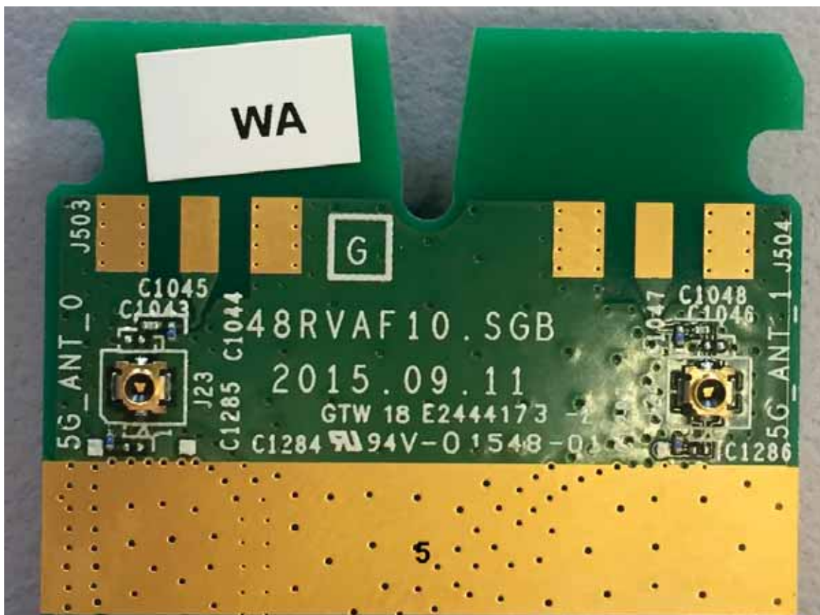
Close-up of Bottom Section Marked 5 - Antenna Ports
