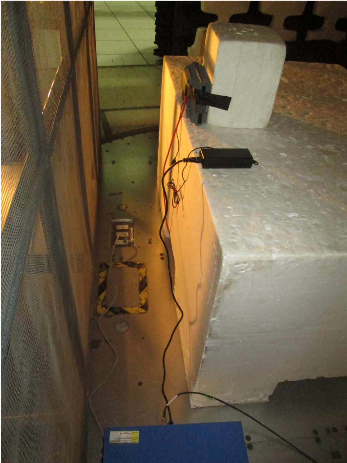
Conducted Emissions Test Configuration Photographs
