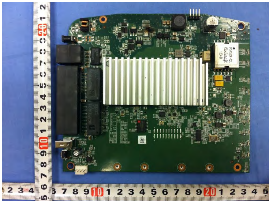
Photo 9 – APINR15P Main Board Front View
