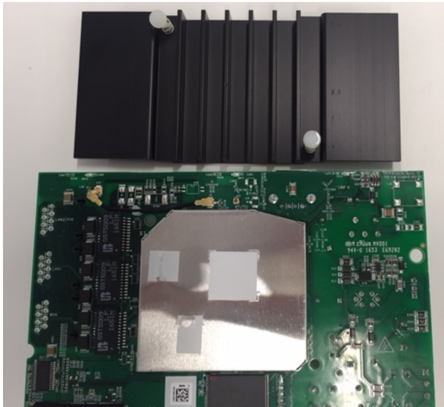
Top View of PCB with Heat Sink Removed
