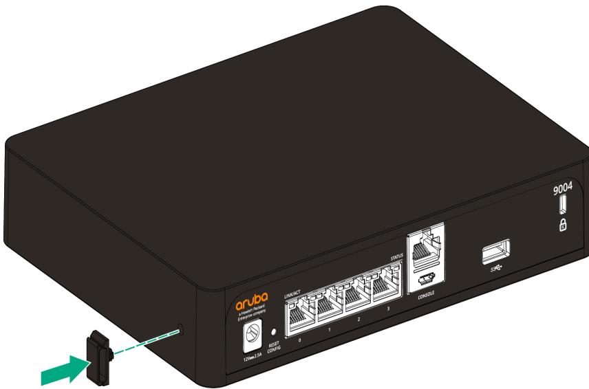
Figure 8 Attaching a cable saddle
