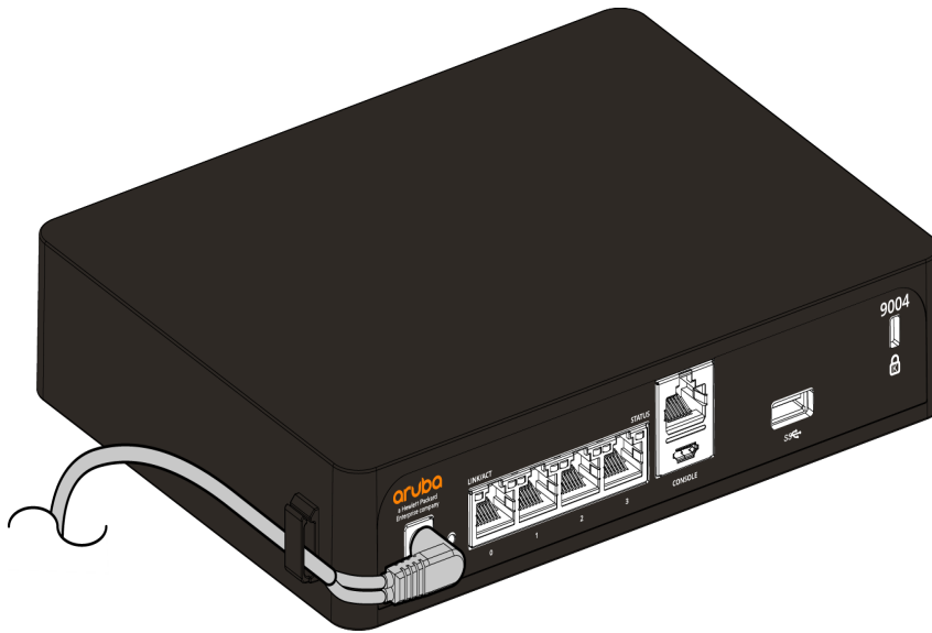
Figure 9 Securing a cable
