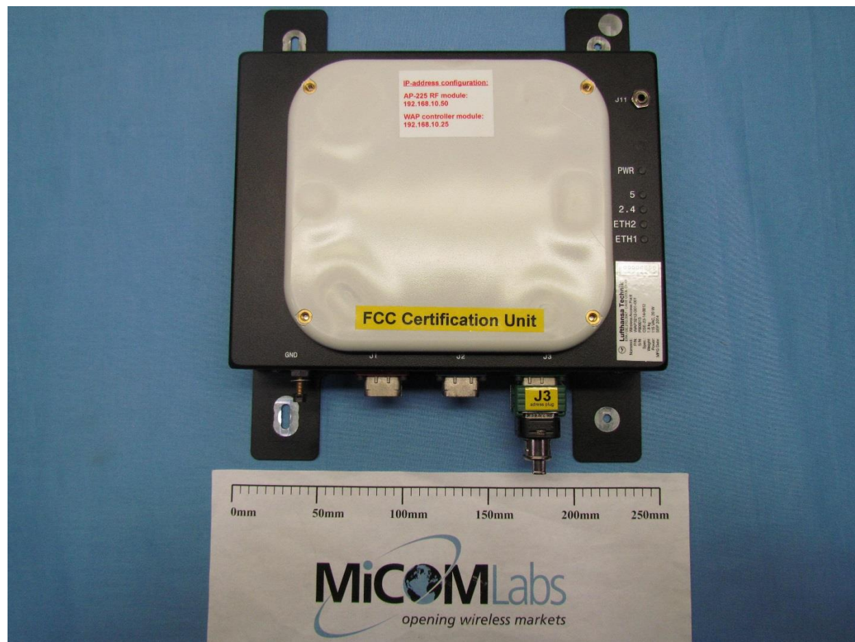
EUT top view – Cabin Wireless Access Point
