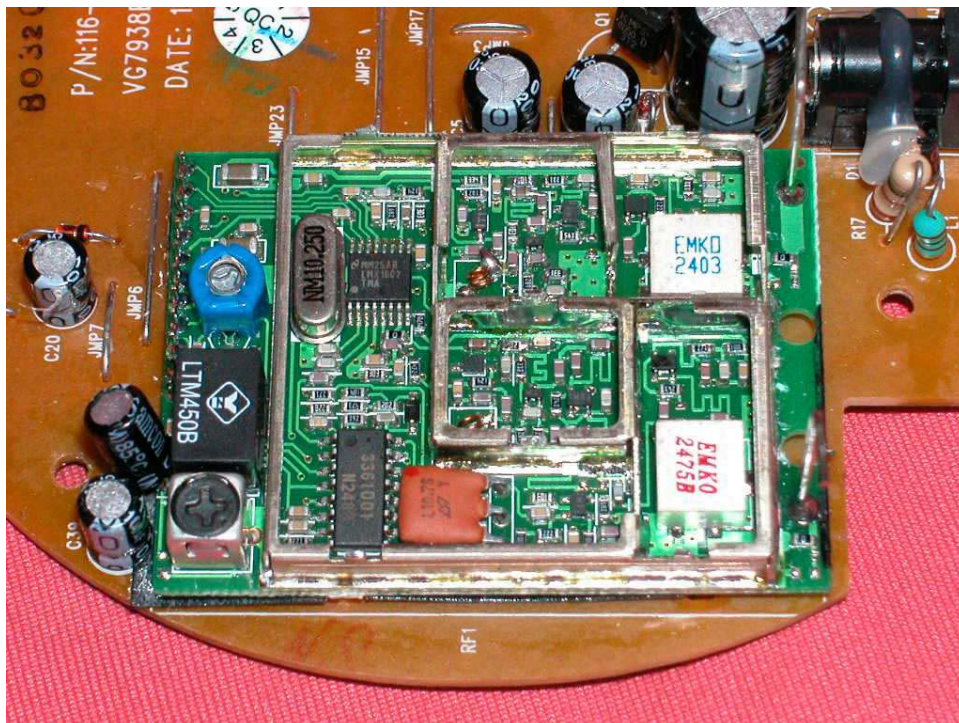
Base Oscillator PCB comp side (View 1)
