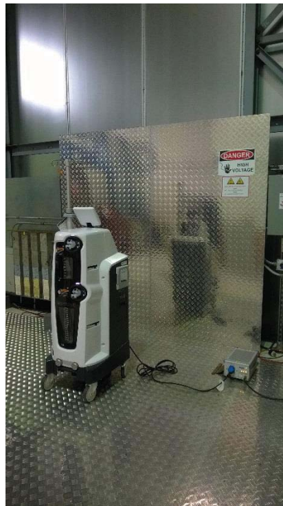
Figure 3.6-2: AC Powerline Conducted Emissions Setup
