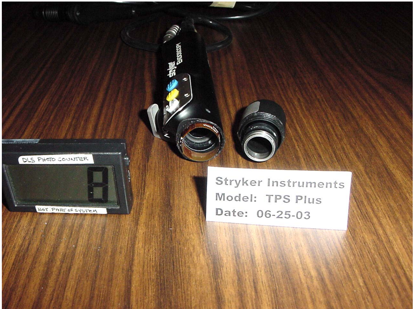
FORMULA SHAVER WITH NOSE PIECE REMOVED, SHOWING ANTENNA
