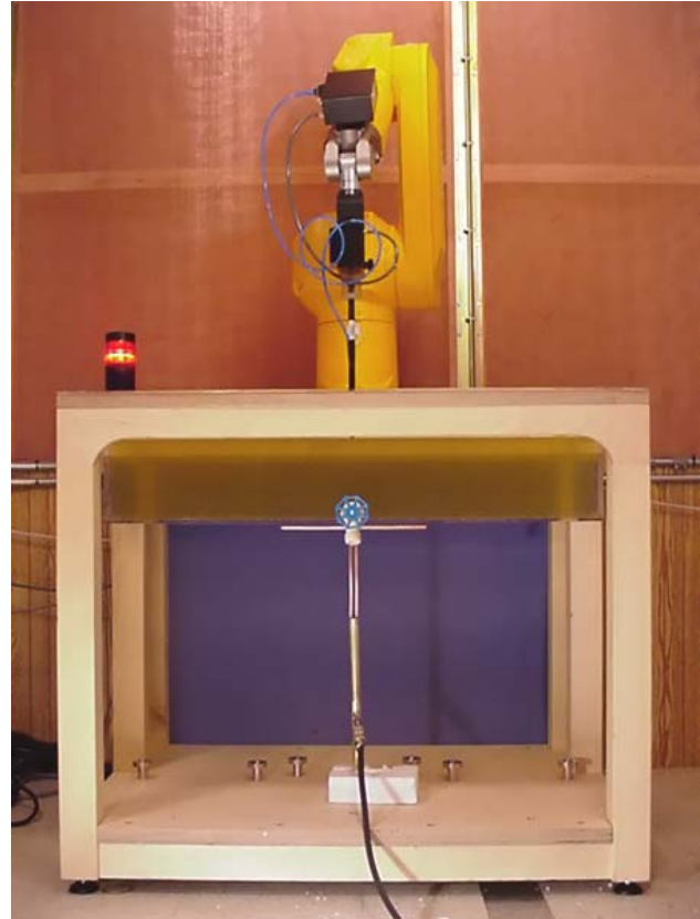
DASY3 SAR Measurement System with validation phantom
