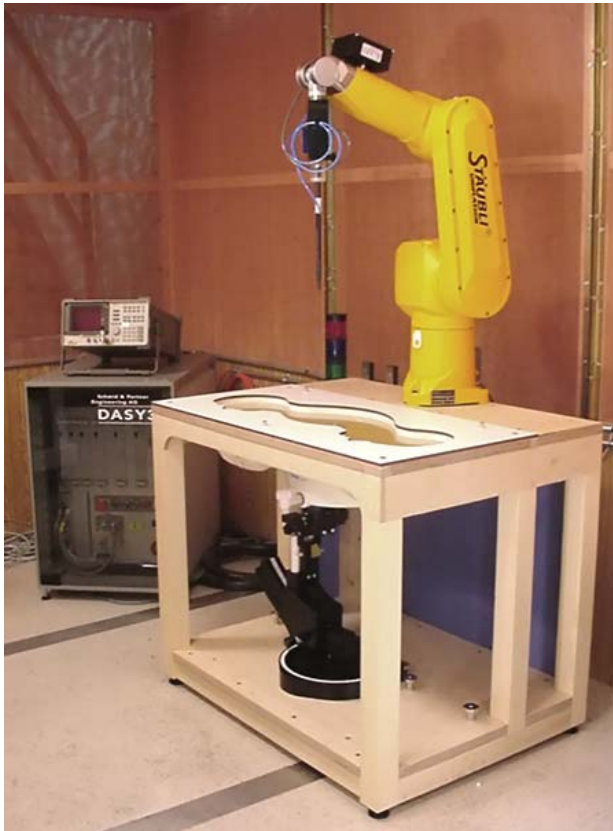
DASY3 SAR Measurement System with SAM Phantom
