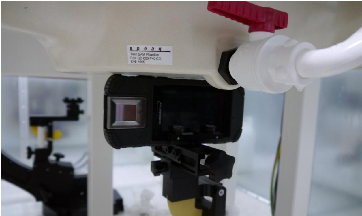
Position 4 EUT right side towards phantom
