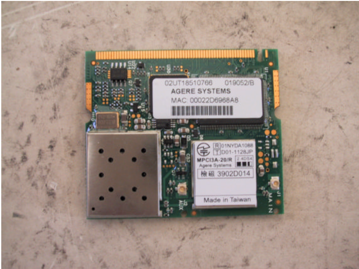
Radio PCB – Top Side
