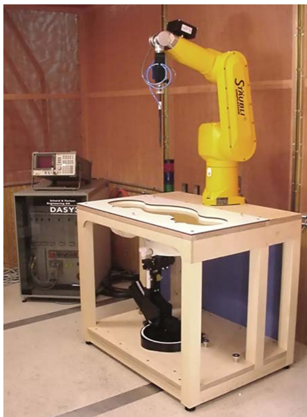
DASY3 SAR Measurement System with SAM phantom
