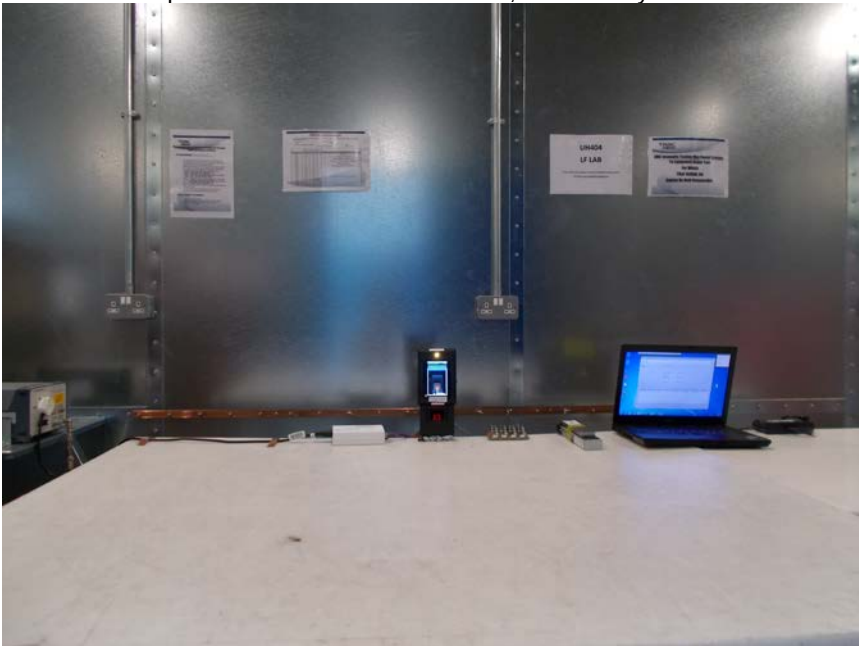
AC power-line conducted emissions, Powered by POE
