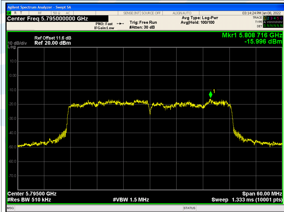
PSD NVNT ac40 5795MHz Ant1
