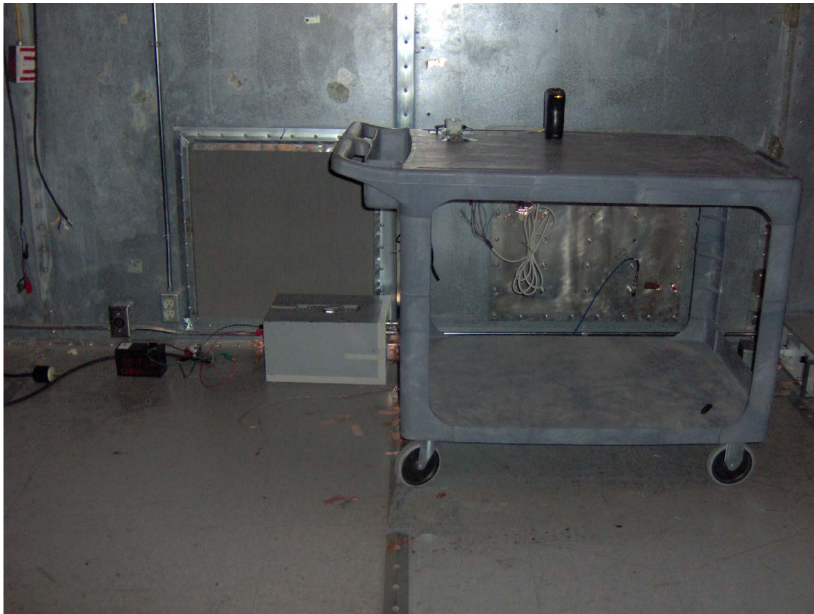
Photo #1: Powerline Conducted Emission Measurements
