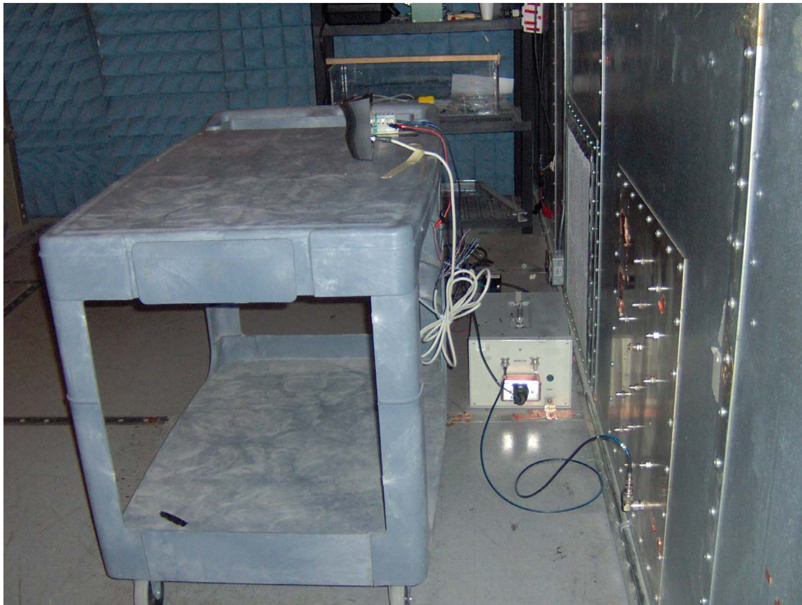
Photo #2: Powerline Conducted Emission Measurements
