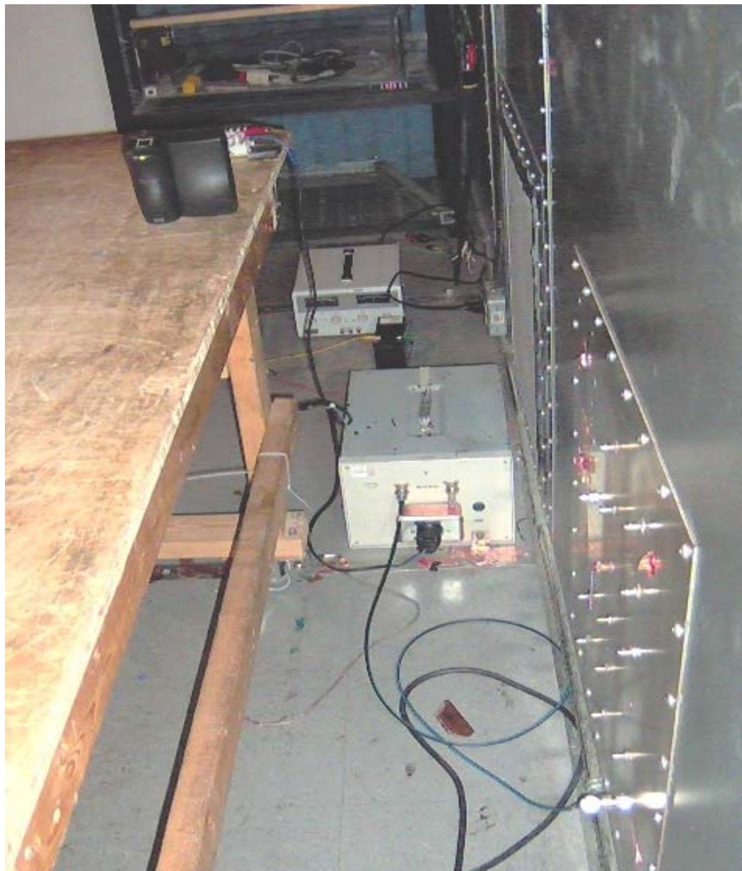
Photo #2: Powerline Conducted Emission Measurements
