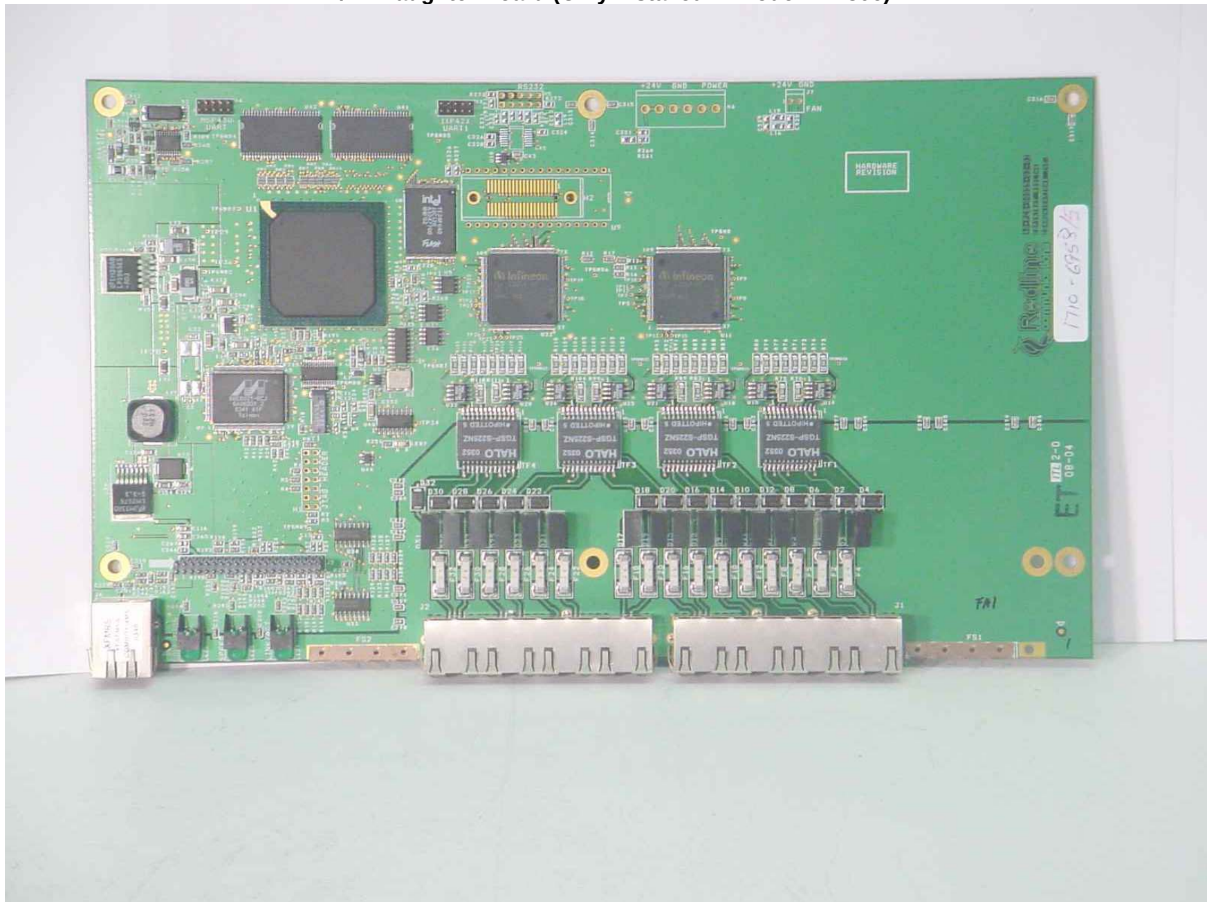
T1/E1 Daughter Board (Only installed in Model AN-30e)
