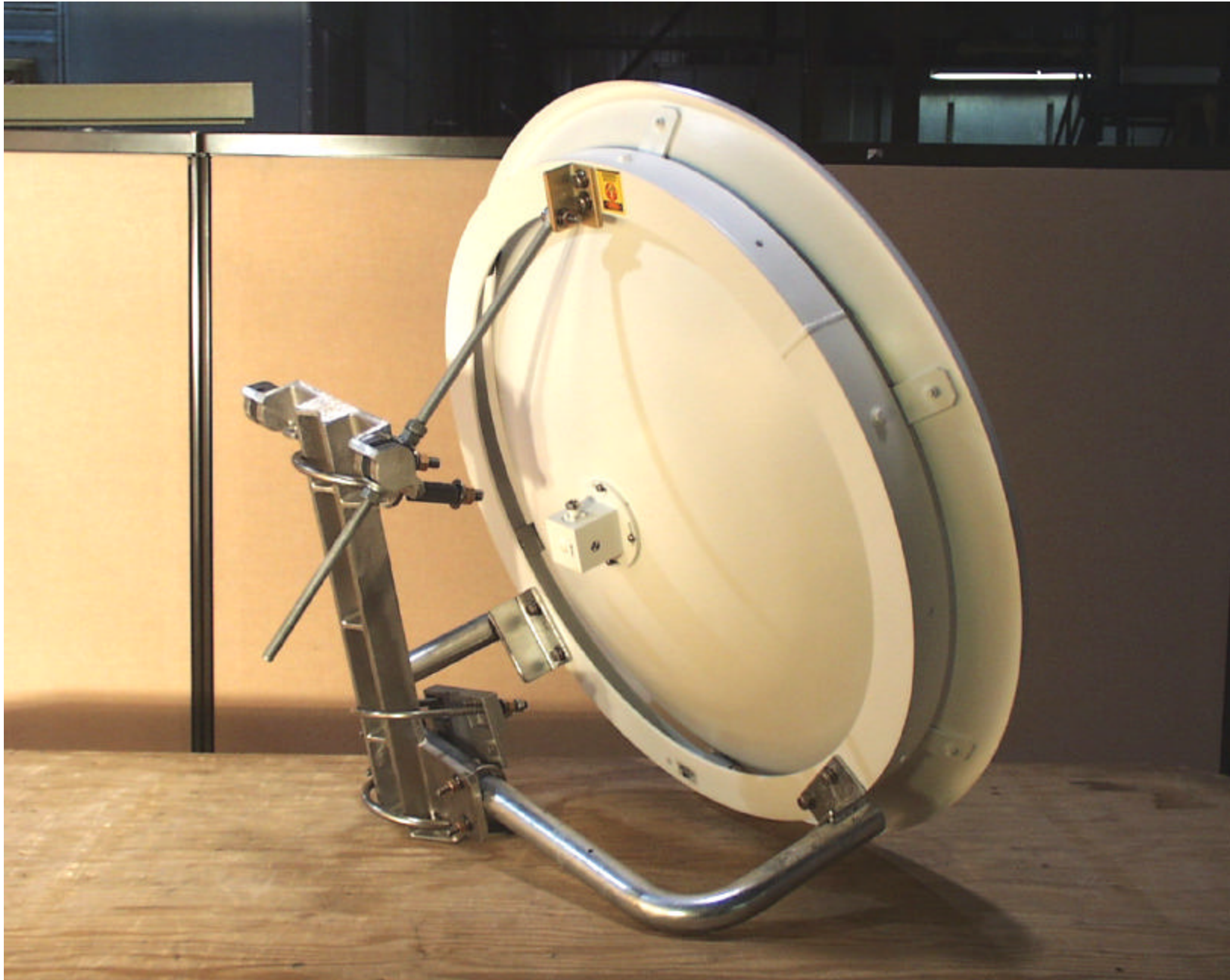
Radiowave Antenna, P/N: SP3-5.2NS, Gain 31.2 dBi (Back)
