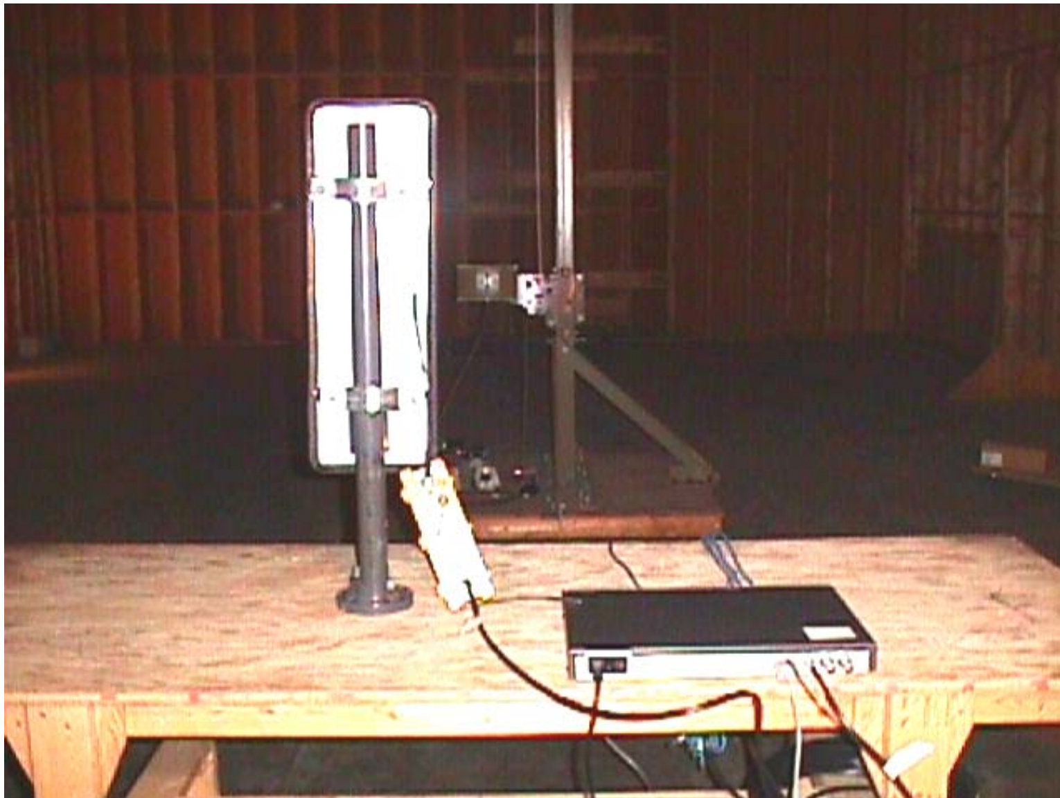
Photo #4: Radiated Emissions Measurements at 3m Distance Radiowave Antenna Model SEC-55V-60-17, Gain: 17 dBi (maximum gain within its family)
