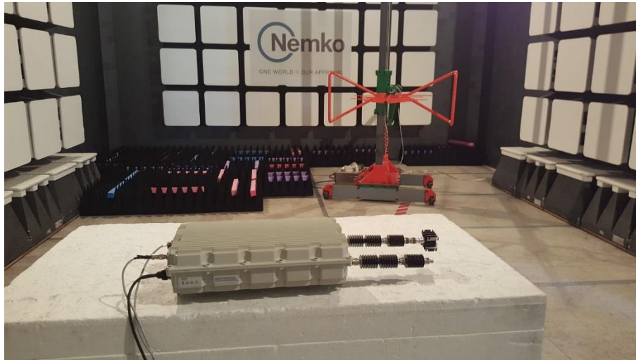
Figure 3.5-1: Test / Measurement Equipment - Set up for Radio Compliance Testing – below 1 GHz
