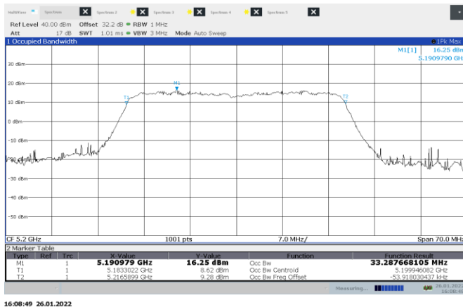
Figure 8.5-5: 99% bandwidth on 40 MHz channel, sample plot
