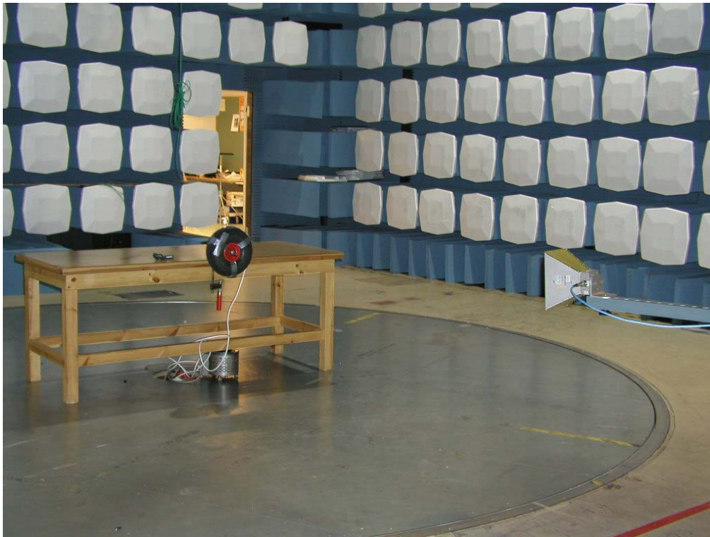
Photograph 1. Radiated disturbance emission test
